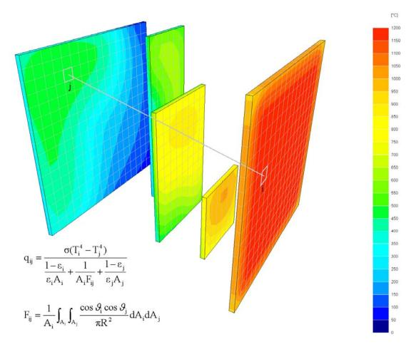
VOLTRA is a thermal analysis program for transient heat transfer in threedimensional rectangular objects.
