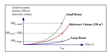
other smoke from fires is assumed to layer itself by plumes, typically towards the ceiling where it creates significantly higher optical densities - and at a later phase of fires when damage is more significant. In the plume-phase all listed detectors of nominal (sensor head) sensitivity rated within typical standards will respond reliably within a narrow time frame, thus not necessitating any response modeling for practical purpose.
