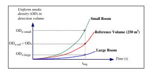
assumed to layer itself by plumes, typically towards the ceiling where it creates significantly higher optical densities, and at a later phase of fires when damage is more significant. In the plume-phase all listed detectors of nominal (sensor head) sensitivity rated within typical standards will respond reliably within a narrow time frame, thus not necessitating any response modeling for practical purpose.
